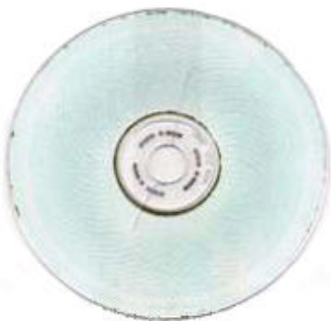
Example of processed CD-R Data has been completely destroyed
