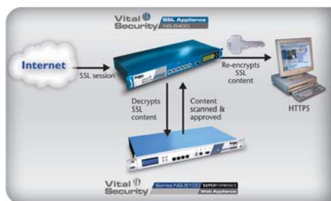
Decryption and scanning of SSL content with Finjan Vital Security Web and SSL Appliances
