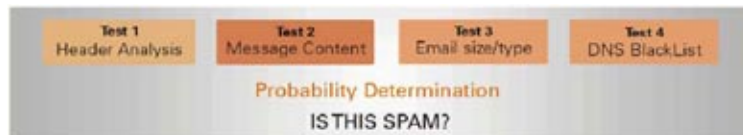
Figure 4. The SpamCensor combines multiple tests to arrive at a spam “score”
