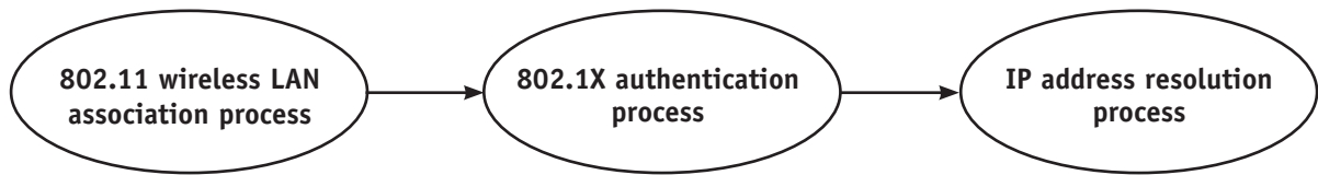
Figure 2: typical WLAN client login process
